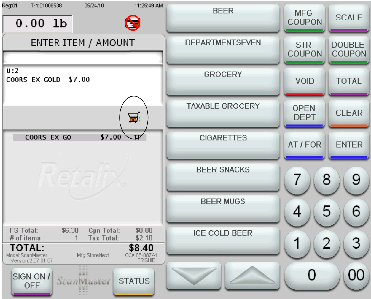
Figure 2 The LaneHawk system has detected an item on the bottom of the basket
