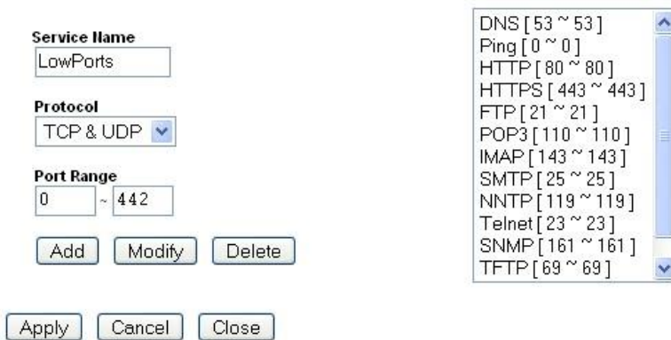
Figure 62 - Firewall Service Configuration
