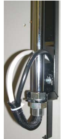
Cut the tie wraps and disengage the cables from the Station
