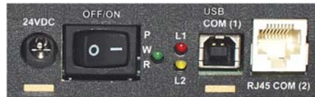
Power switch location
