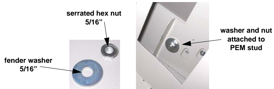
Figure 3.47 Fender (oversized) washer and serrated hex nut
