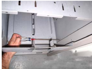
Figure 3.48 Tightening the rear M5 screws from inside the robot
