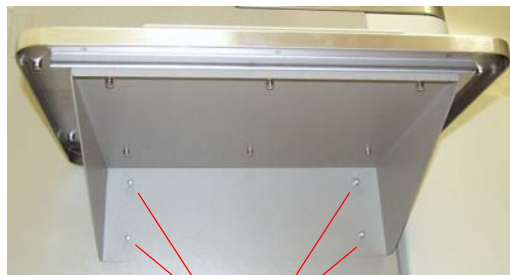
Four M5 screws secure the Side Assist shelf to the Station
