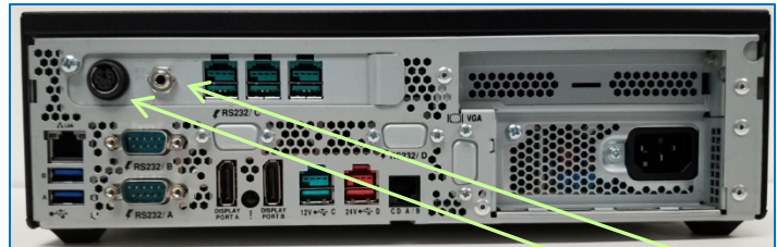
Reduced I/O pictured here with the additional PS/2 and Line-Out ports added (optional). The 3 P-USB ports are at the top.
