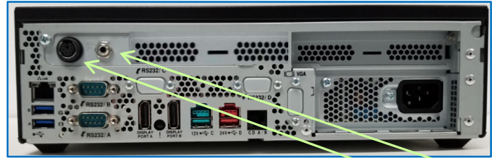
Base I/O pictured here with only the additional PS/2 and Line-Out ports added (optional). A blank plate covers the Upper Row area.
