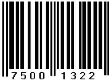
Figure 9-12: Sample Short 8-digit EAN code
