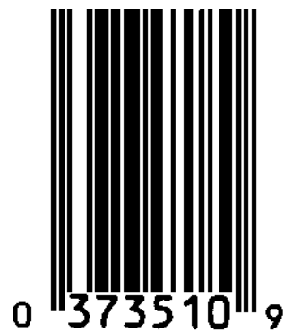
Figure 9-10: Sample Short 6-digit UPC-E Code
