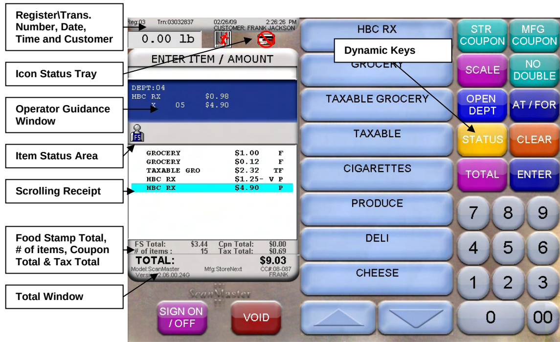
Figure 9-1: DynaKey Operator Display
