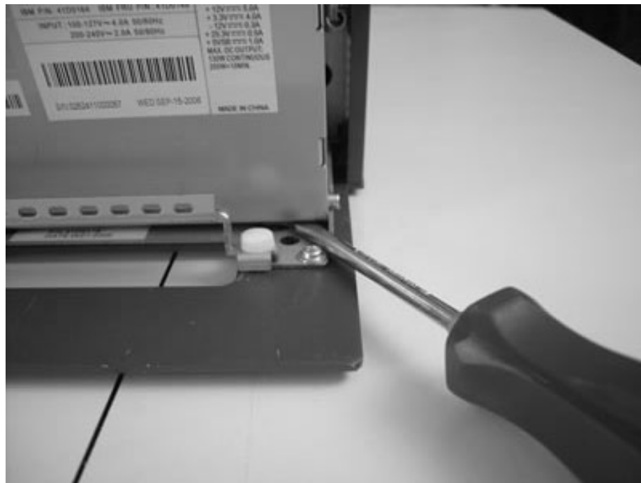
Figure 55. Placement of the screwdriver to remove the power supply
