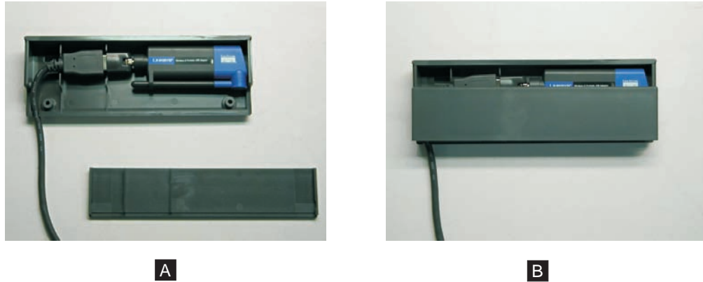
Figure 18. Assembling and installing the wireless adapter
