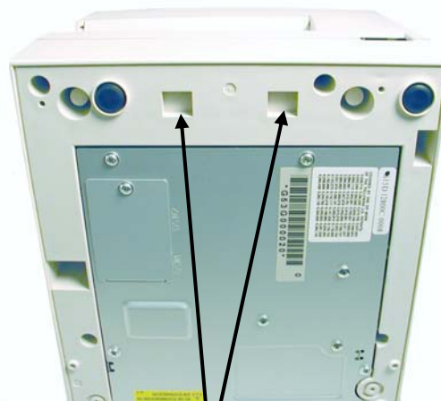
Notches on underside of DT50 Series Printer
