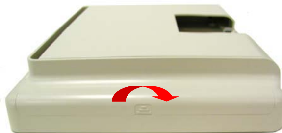
Figure 5-21. Removing the LCD Side Panel
