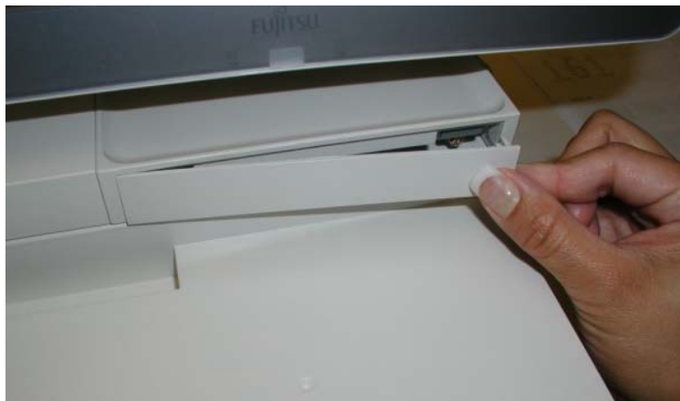
Figure 5-20. Installing the Face Plate
