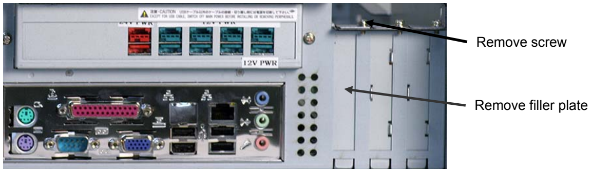
Figure 7-24. Removing the Filler Plate from the Back Panel
