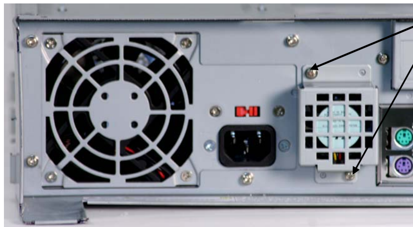
Figure 7-33. Replacing the Fan
