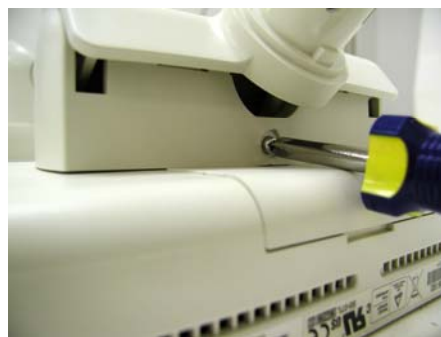
Figure 5-32. Attaching the Tilter
