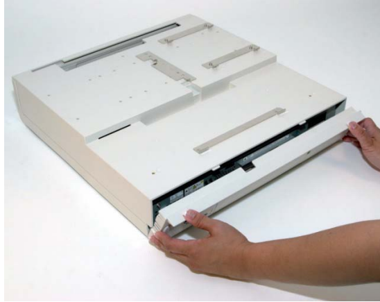
Figure 7-4. Removing the Front Panel
