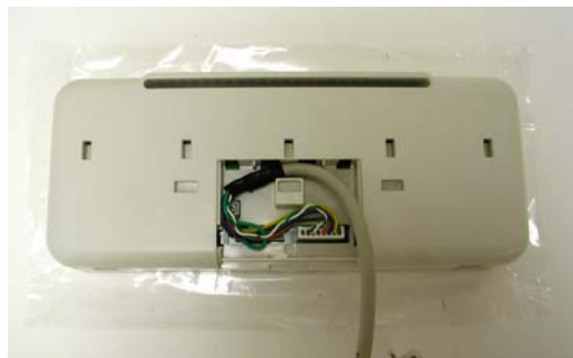
Figure 5-30. Connecting the USB Connector
