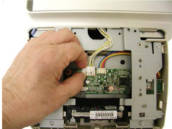
Figure 5-25. Attaching the MSR Connector
