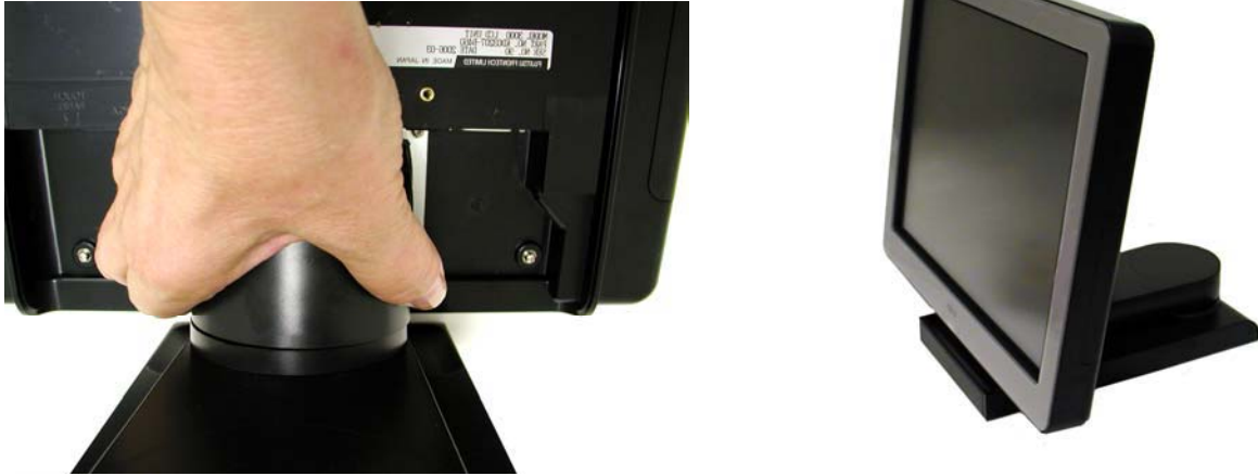
Figure 5-16. Attaching the Hinge Cap
