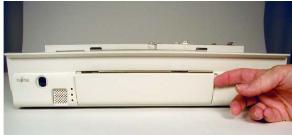
Figure 7-2. Opening the Controller Front Door
