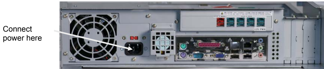
Figure 5-51. Connecting AC Power
