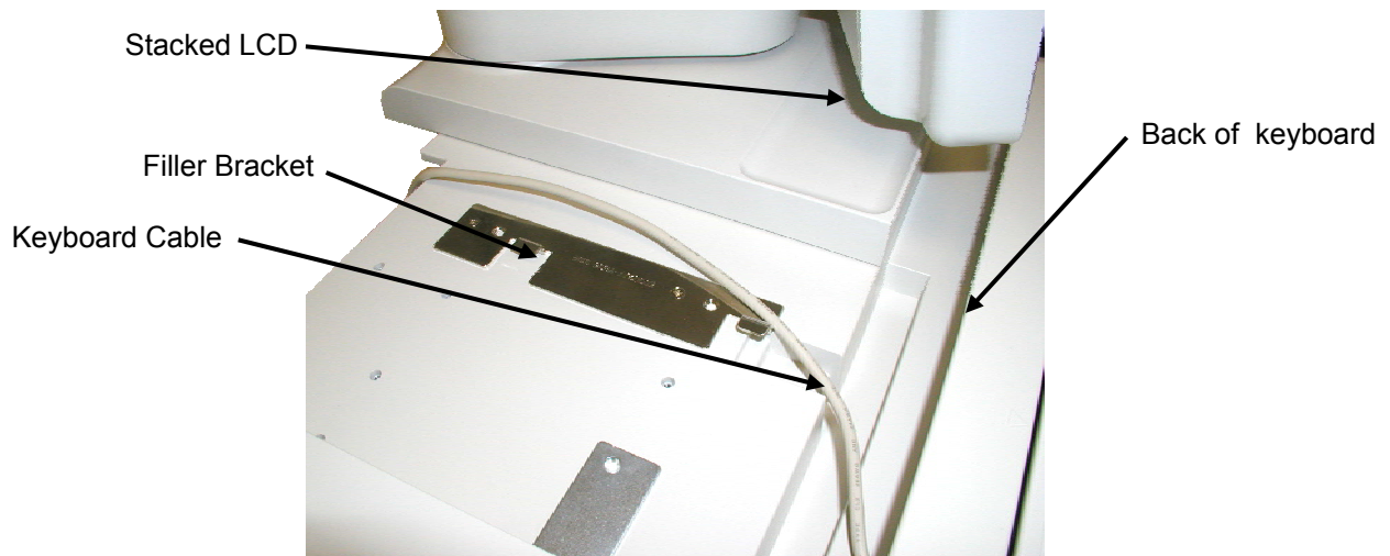
Figure 5-39. Putting the Keyboard on the Controller
