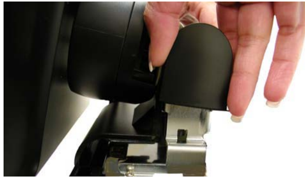
Figure 5-14. Replacing the Top Hinge Cover
