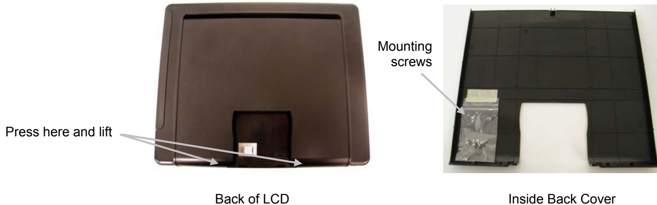
Figure 5-10. Removing the LCD Back Cover
