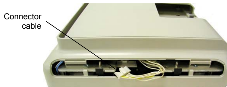
Figure 5-22. Accessing the Connector Cable
