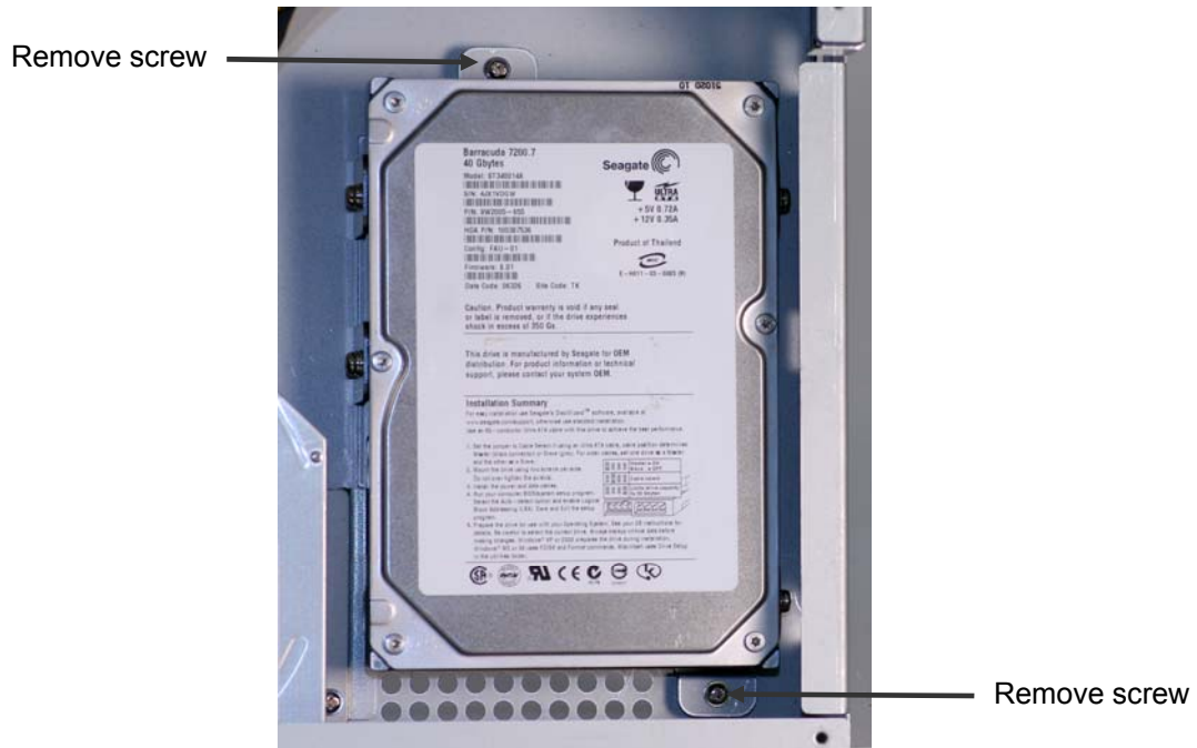
Figure 7-21. Removing the Hard Drive from the Chassis
