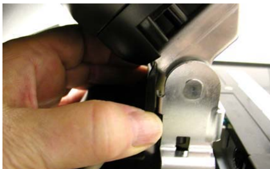
Figure 5-6. Removing the Bottom Hinge Cover
