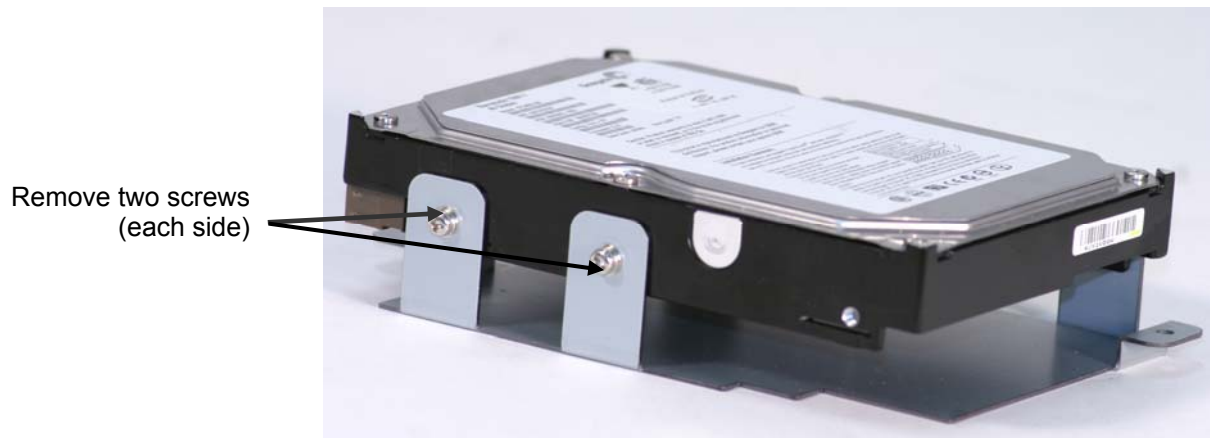
Figure 7-22. Removing the Hard Drive from the Bracket
