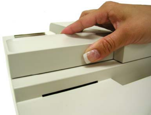
Figure 5-45. Installing the Front Filler Panel
