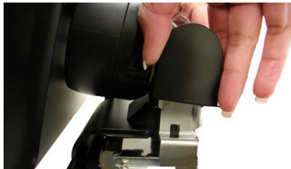
Figure 5-5. Removing the Top Hinge Cover
