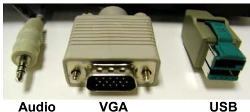
Figure 5-9. VGA Cable Configuration with Optional Audio Cable
