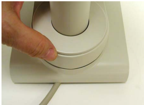
Figure 5-37. Fitting the Collar into Place
