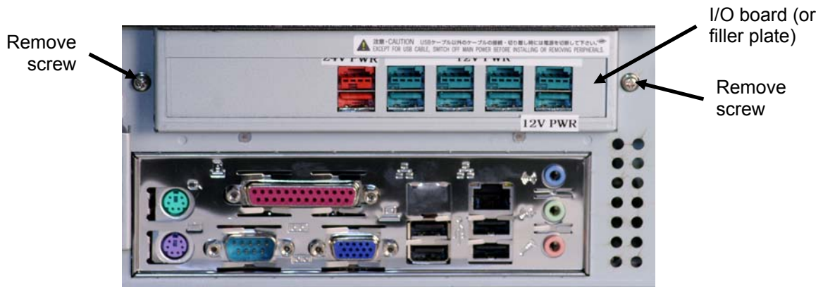
Figure 7-26. Installing the I/O Board
