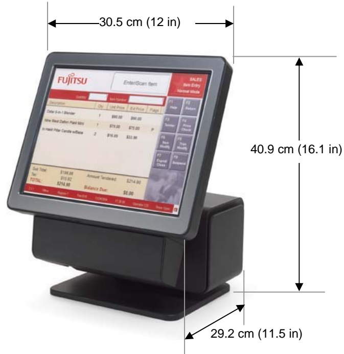
Figure 3-1. TP3000 XT Dimensions (for units with 12.1" LCD)
