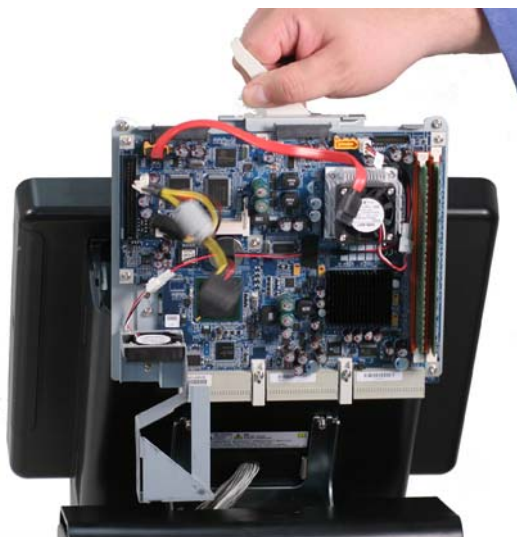
Figure 7-3. Removing the Motherboard
