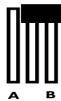
LK2 Jumper Position for Scale Range of 150 lbs. (Stationary or Solo Bag Scale)
