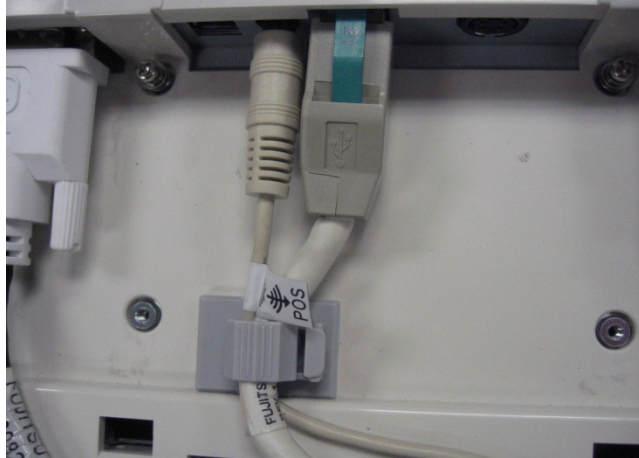
Correct Installation with Strain Relief
