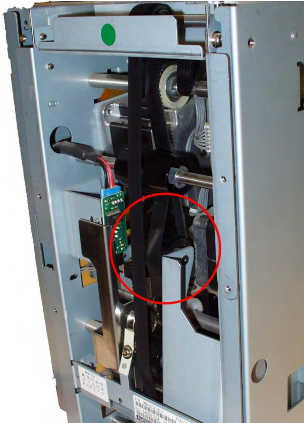
F53 Rear Belt in Wrong Position
